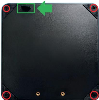
**Figure 1** – Shows the **location of screws** securing the back panel to the Mini PC, along with the **pull-out tab** for panel removal.
