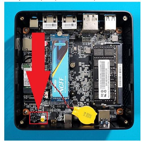
4. Using small tweezers, gently remove the black plastic pin header from its current position. Move the header to bridge pins 2 and 3, enabling the auto power-on feature.
